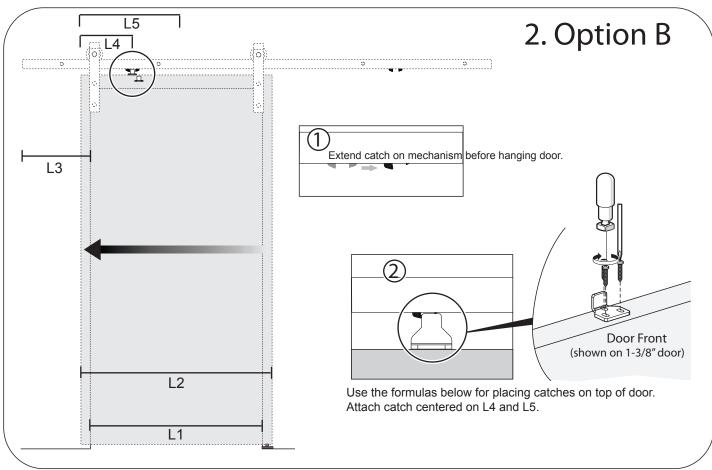
Note: This method centers the door over the opening and also allows for enough overlap for the floor guide to always engage the door.
