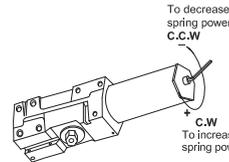
Adjust spring power DO NOT exceed the maximum turns in either direction!
