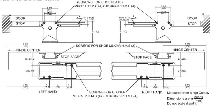
BEFORE INSTALLING MOUNTED STOP FACE (PARALLEL ARM), TURN BACK CHECK SELECTOR VALVE (FOUND IN OPPOSITE SIDE OF CLOSER FROM REGULATING SCREWS SIDE) ALL THE WAY IN (CLOCKWISE)!
