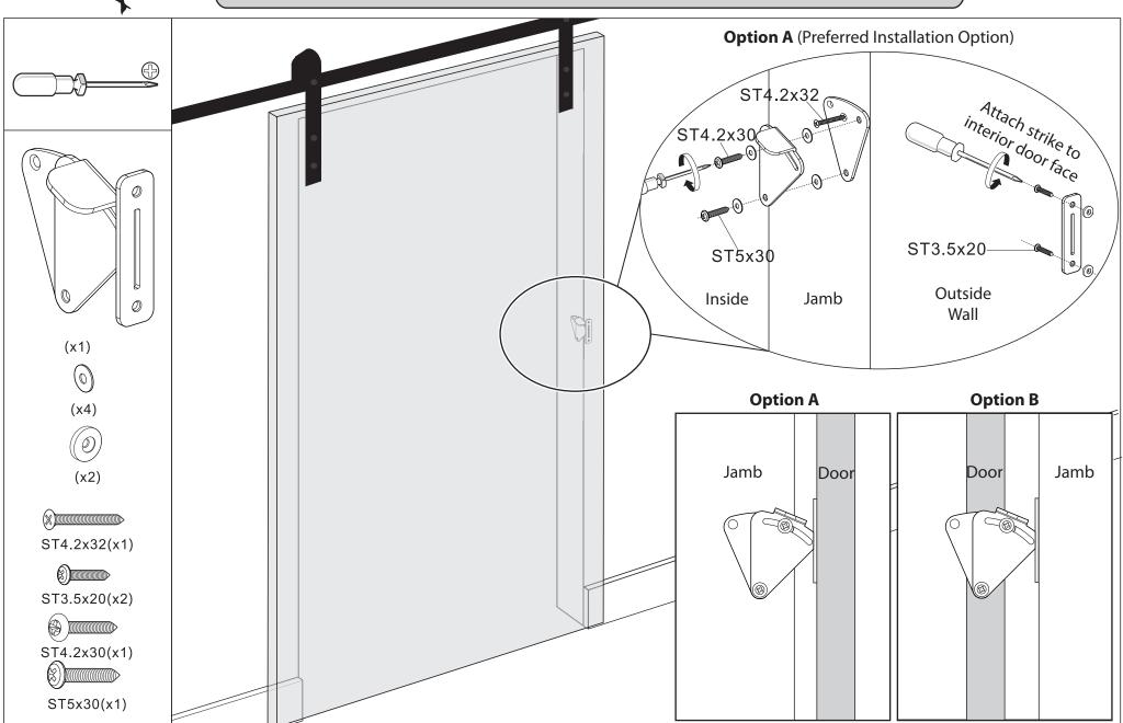
For emergency egress, slide a thin card such as a credit card upward to release the lock. Warning: if used on a pocket door, a 1/8" diameter through-hole must be drilled behind the strike plate so that an object such as a paper clip can release the lock.
