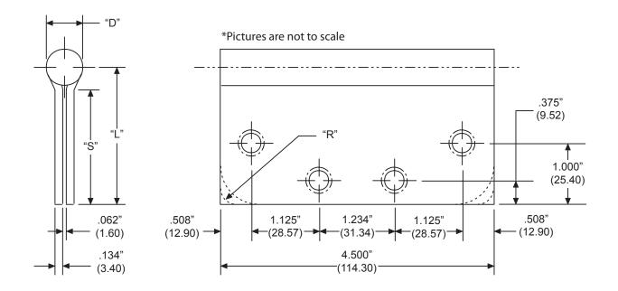
COM4545 hinges are Standard Duty COM4545BB (Ball Bearing) hinges are Heavy Duty Made of Steel Available in US26D and US10B
