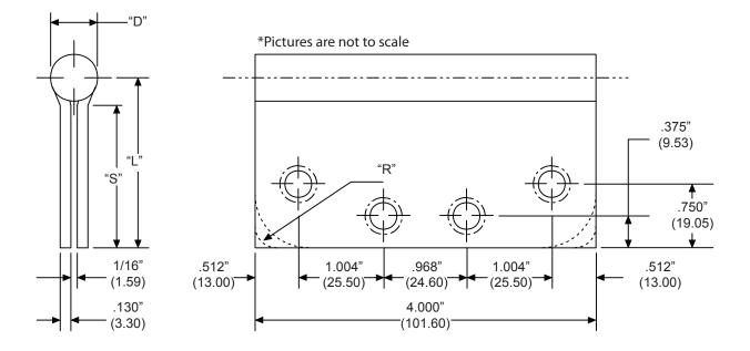
COM4040 hinges are Standard Duty Made of Steel Available in US26D, US15, and US10B
