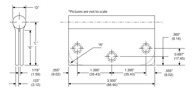
COM3535 hinges are Standard Duty Made of Steel Available in US26D, US15, and US10B
